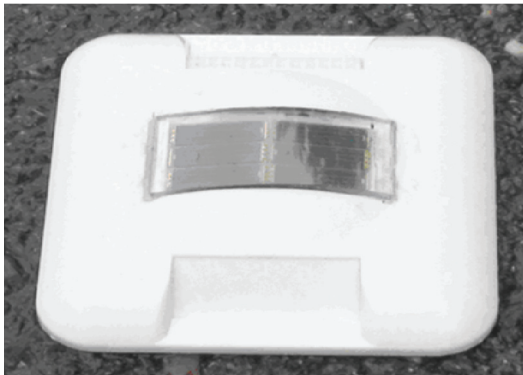
Figure one: The wireless and batteryless traffic sensor based on GMR. The device is approximately 4x4 inches with thinness of 20mm.
